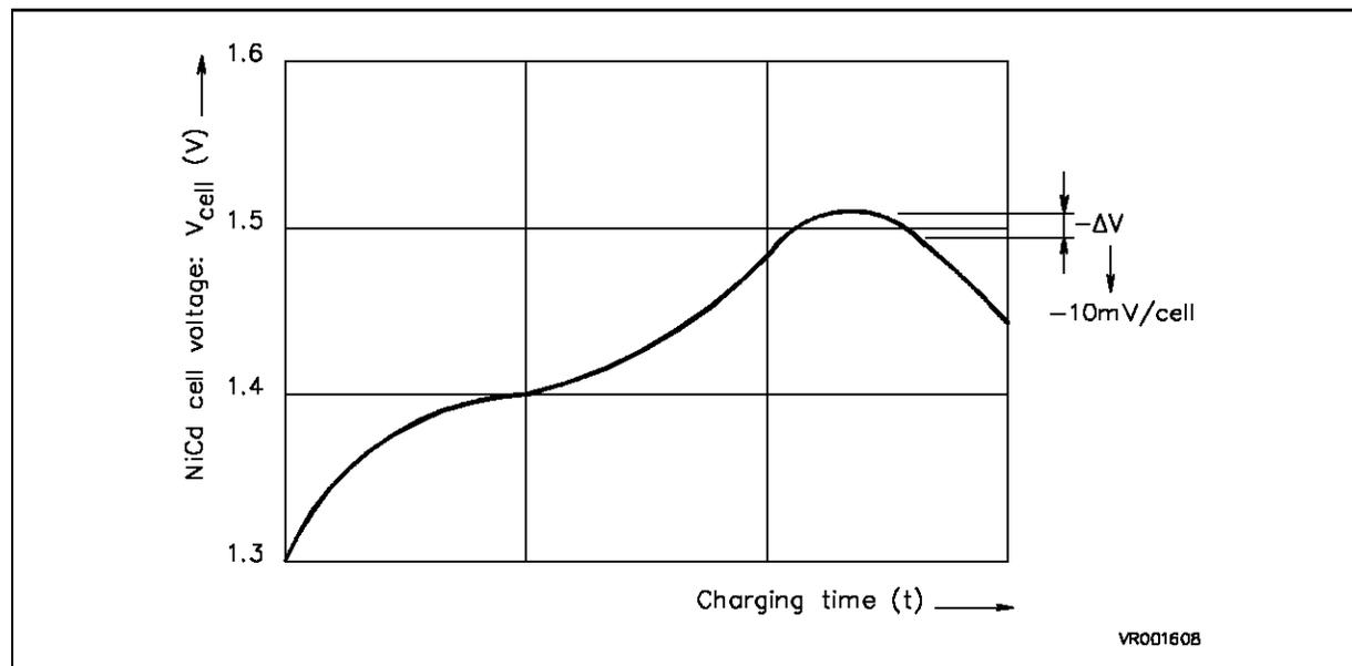
When a NiCd battery reaches full charge, its voltage decreases slightly (Figure 2). The negative delta voltage method ( $-\Delta V$ ) consists of stopping the charge as soon as the voltage characteristic slope becomes negative. This technique allows the very rapid charge of a NiCd battery, near to its full capacity. Moreover, no compensation for the age of the battery is required because only relative voltages are measured.
