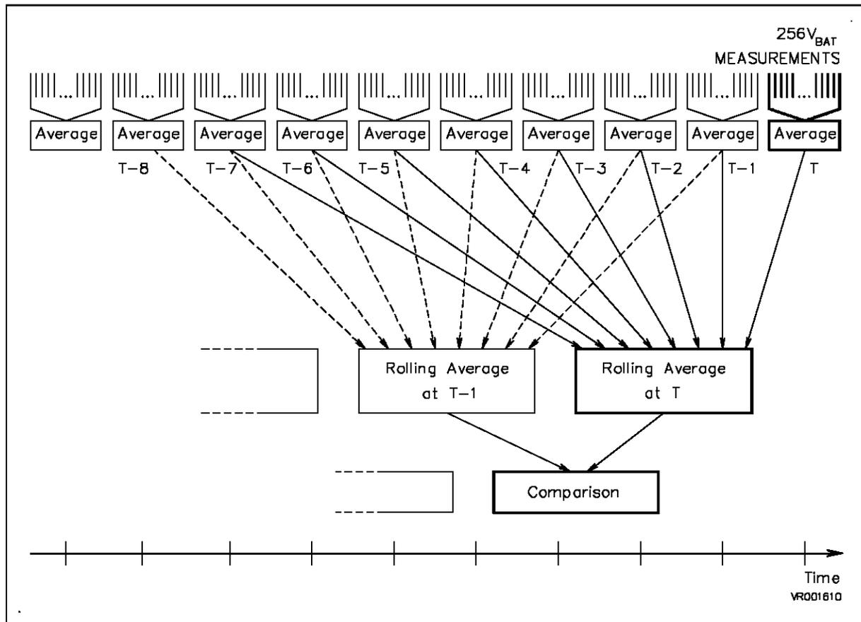
The response time to detect the battery voltage drop ranges from 1 to 8 seconds, depending on the slope of the battery voltage curve at the charge completion. A longer delay time is able to increase the noise immunity, but at the cost of an extended response time.
