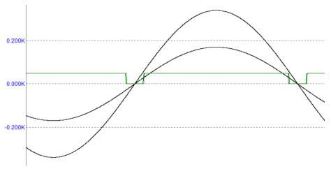
Sometimes you don't need to monitor the mains itself, but you need to monitor a controlled mains load. Also here the ZC circuit come in handy. An example is shown in Fig 2. Here a triac controls an incadescent bulb either on or off. With the help of the ZC you can monitor a shorted load, an open load, missing live voltage, and also that the triac is working properly. "
