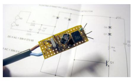
Transistor Q1 stays off during the majority of the mains cycle, during which C1 is charged via R1-R2 and D5. Q1 turns on and feeds current from C1 to the opto via R4, whenever the mains voltage (divided by (R1+R2)/R3) is lower than the voltage across C1. The voltage across C1 will reach within about 400ms an equilibrium that defines the final operating point. The voltage across C1 never exceeds 10 volts with the given resistor ratios. The voltage stabilizes at a point
