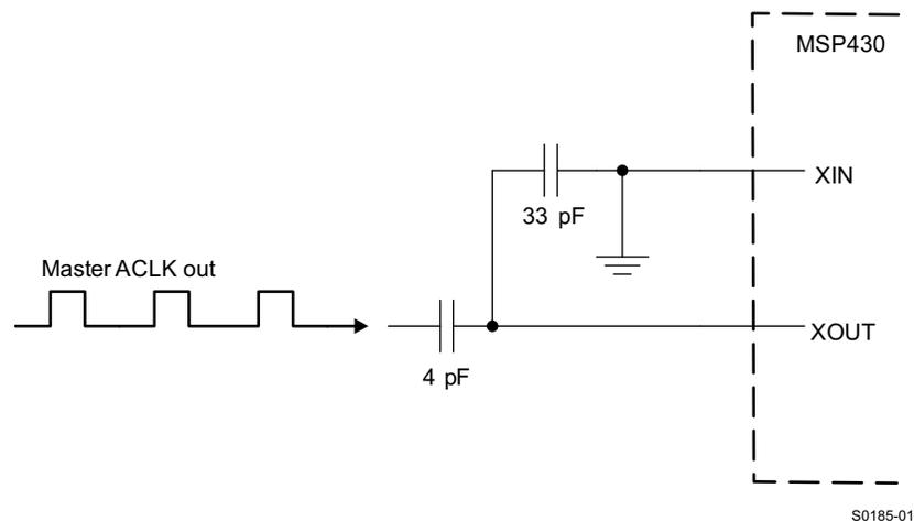
**Figure 2. Slave ACLK Input Schematic**
