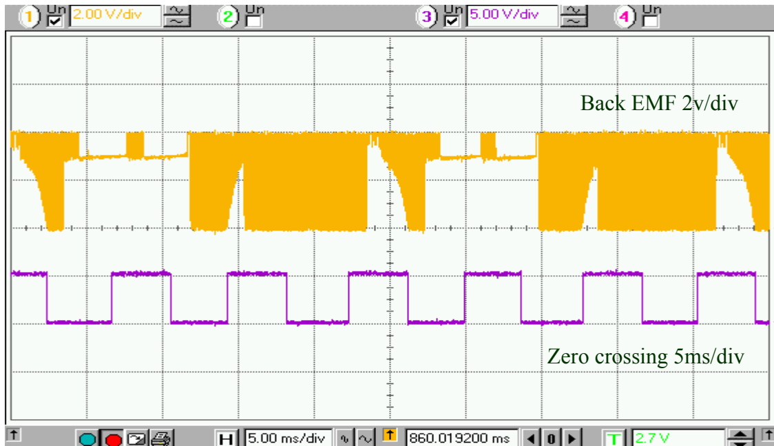
Fig.3.9 Improved zero crossing detection by pre-conditioning circuit.
