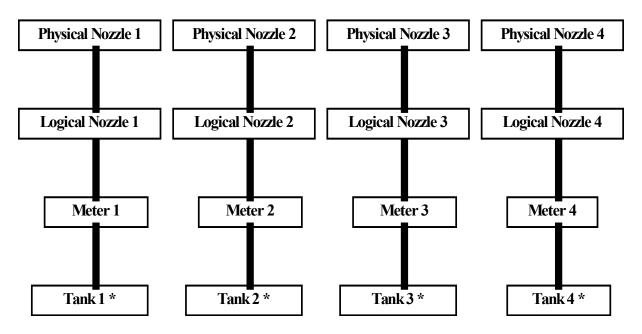
In this example a MPD is configured with 4 grade options. Each grade option has a direct relationship with its own meter, logical nozzle and physical nozzle. This dispenser does not support blending.
